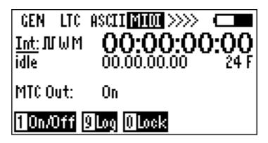
Changes the status of the midi timecode (MTC) generator. In this first software version the MTC generator is locked to the main timecode generator at all times. In future software the MTC in will be activated as well as the possibility to run the MTC generator at a different frame rate from the main LTC generator allowing a gearbox function.
