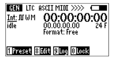
In this menu the timecode generator parameters can be set. The generator starts from 00:00:00:00 and can be set from the following sources.
